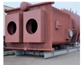
Combined water tube and shell boiler
