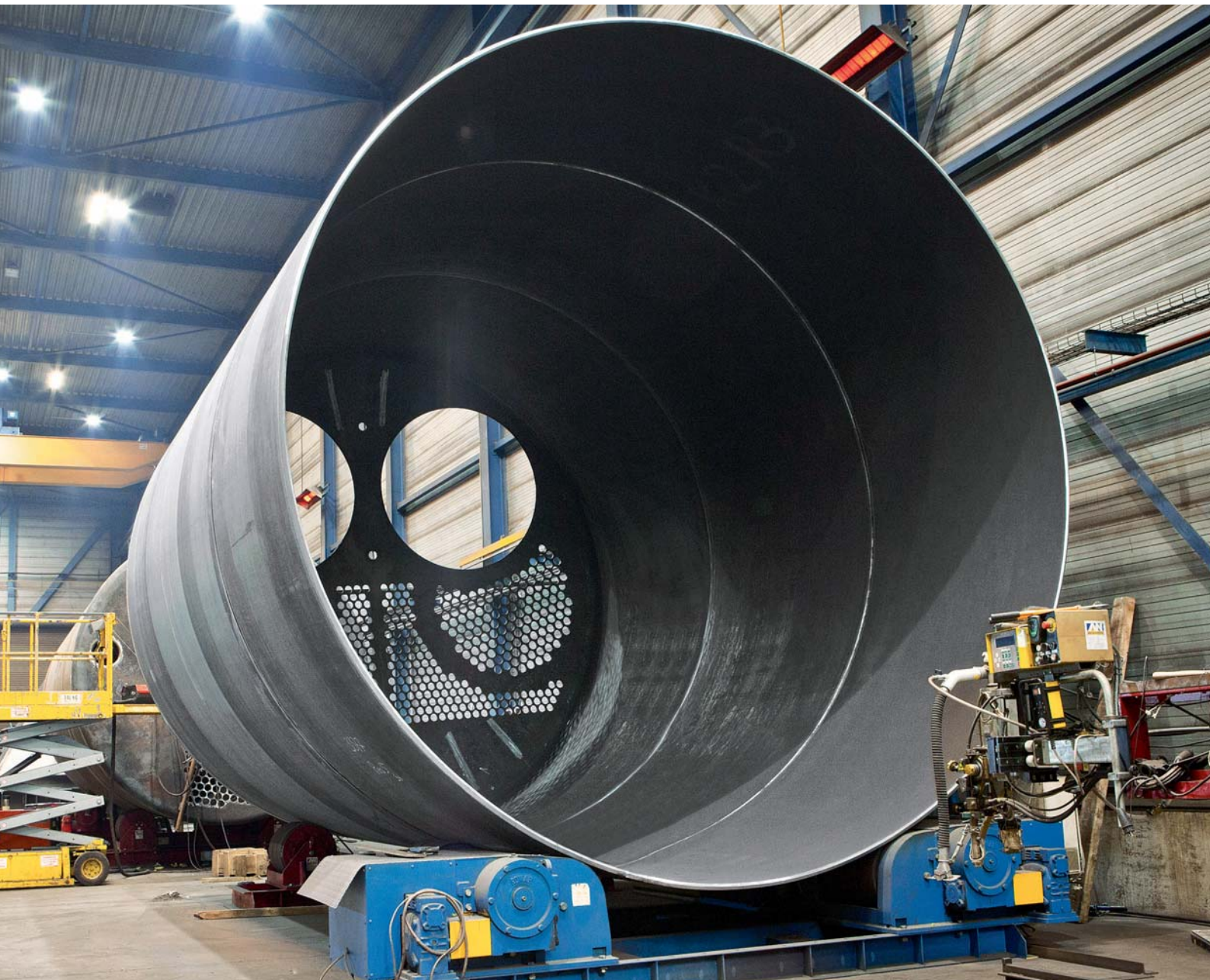
Double flame tube boilers being manufactured at HKB's facility in Venlo, Holland.
